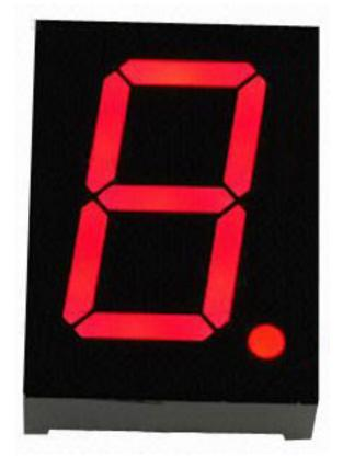
Each of the LEDs in the display is given a positional segment with one of its connection pins led out from the rectangular plastic package. These LED pins are labeled from "a" through to "g" representing each individual LED. The other LED pins are connected together forming a common pin. So by forward biasing the appropriate pins of the LED segments in a particular order, some segments will brighten and others stay dim, thus showing the corresponding character on the display.
