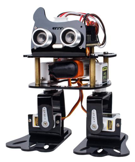
This cute learning kit focuses on the popular open source platform Arduino. You can learn the knowledge of the Arduino servo and ultrasonic ranging module by applying this kit.
