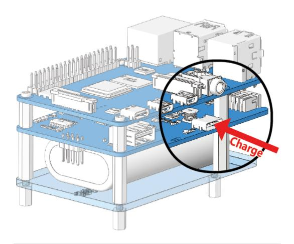
**Warning:** When you put the battery in for the first time or when the battery is unplugged and put in again, the battery will not work properly, at this time, you need to plug the Type C cable into the charging port to turn off the protection circuit, and the battery can be used normally.
