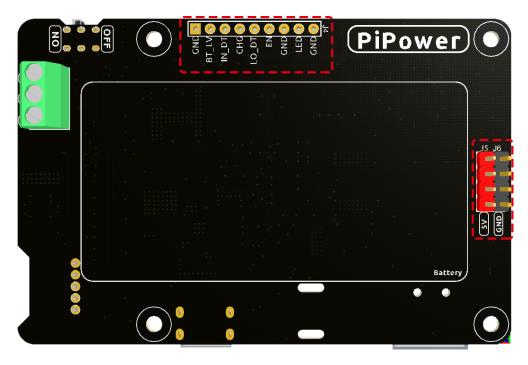
In order to meet the DIY needs of customers, multiple signal pins are provided on the PiPower, but they are not soldered by default.
