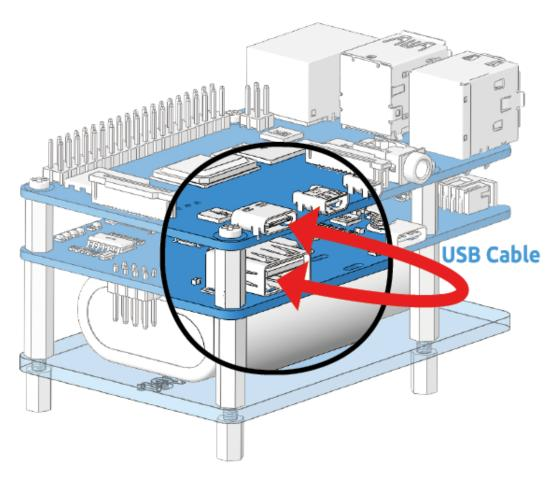
8. PiPower needs to be activated with the USB-C cable at the charge port the first time you use it or re-plug the battery
